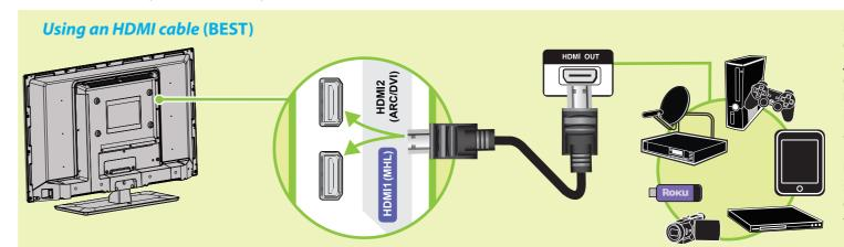
Multipurpose jacks: You can plug any device that uses HDMI into any HDMI jack. However, certain devices must be connected to the **HDMI1 (MHL)** or HDMI2 (ARC/DVI) jack. See the instructions that came with your MHL, ARC, or DVI device for more information.
